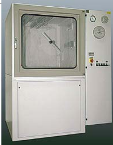
A Typical Dust chamber
