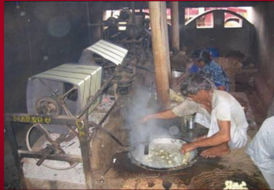
Efficient ovens in silk reeling units
