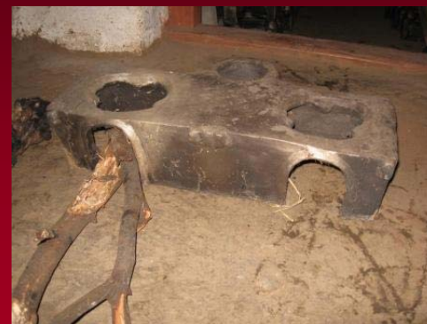
Finished clay stove being tested
