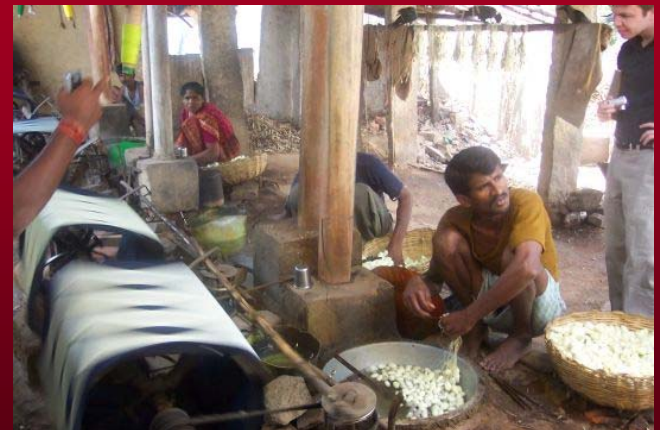
Silk being reeled at a reeling center from the cocoons in the basket at extreme right
