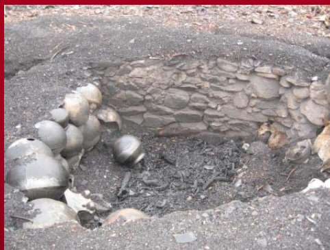
Heat treatment of clay stoves (in open air)
