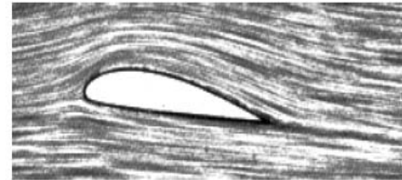
Attached flow around a profile
