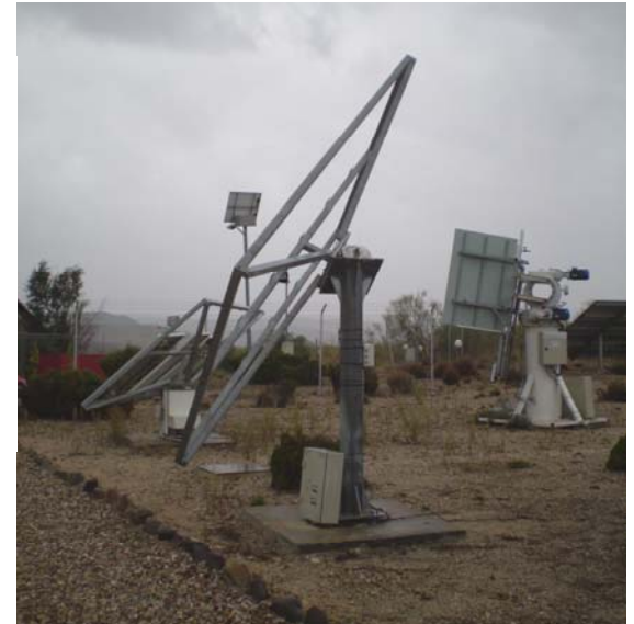
Above: A dual-axis tracker. The 180 degree tracking allows the panels to generate an additional 15% power than the single-axis tracking.
